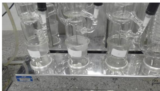
Fig. 6. Initial extraction in Soxhlet with different solvents
