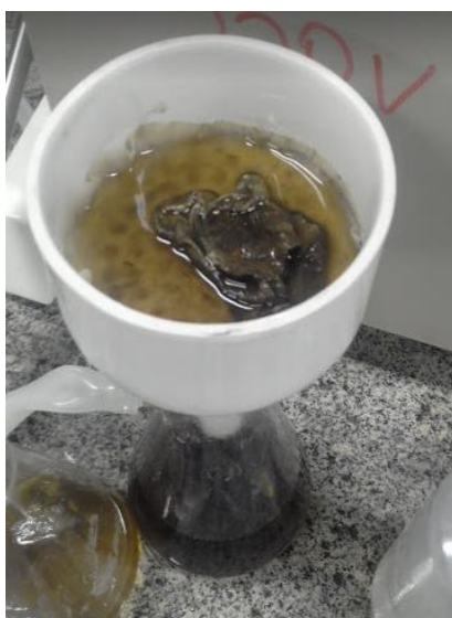
Fig. 3. Vacuum filtration of the fungus in a homemade medium
