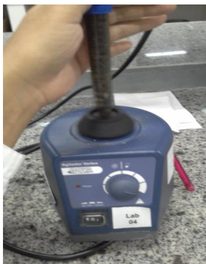
Fig. 4. Realization of the traditional Bead Mill technique
